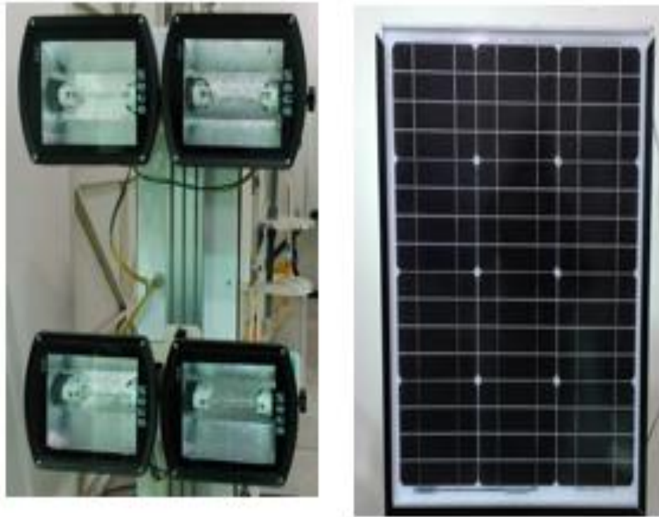
Fig. 1: Halogen Bulbs Using as a Solar Simulator and PV Panel
